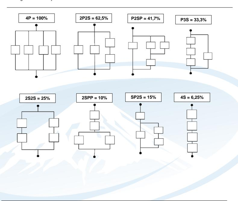
Maximum Cooling Power is the 4P connection, this is the 100% max line
